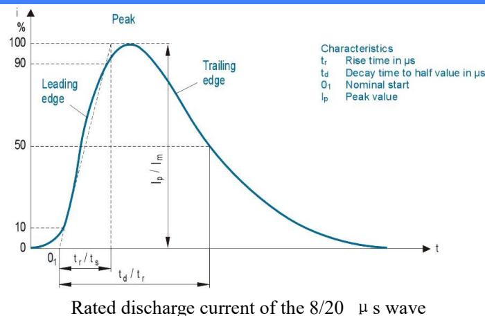
Rated discharge current of the 8/20  $\mu$  s wave
