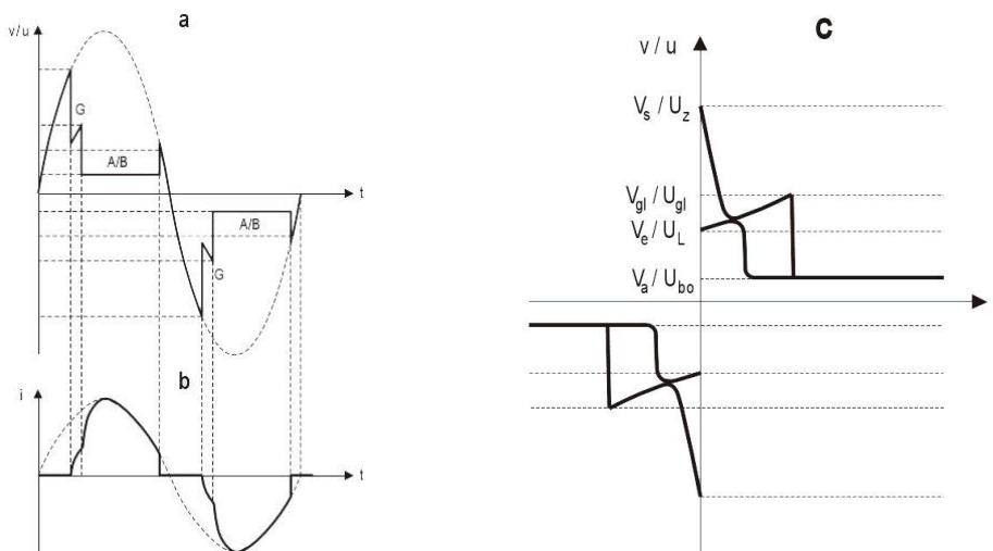
a : shows the voltage curve at the arrester
